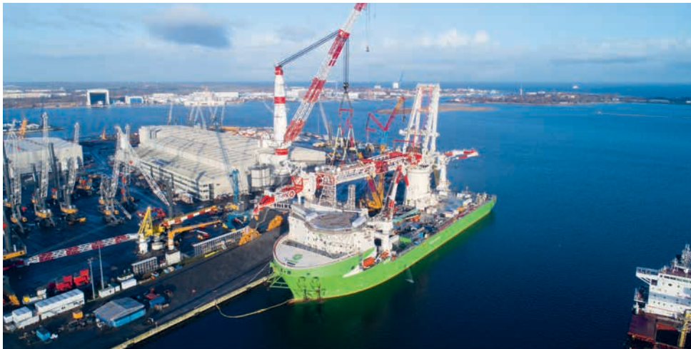
The biggest crane that Liebherr has built to date: the HLC 295000 on the Orion special-purpose vessel. The crane can lift up to 5,000 metric tons with an outreach of 35 meters.
