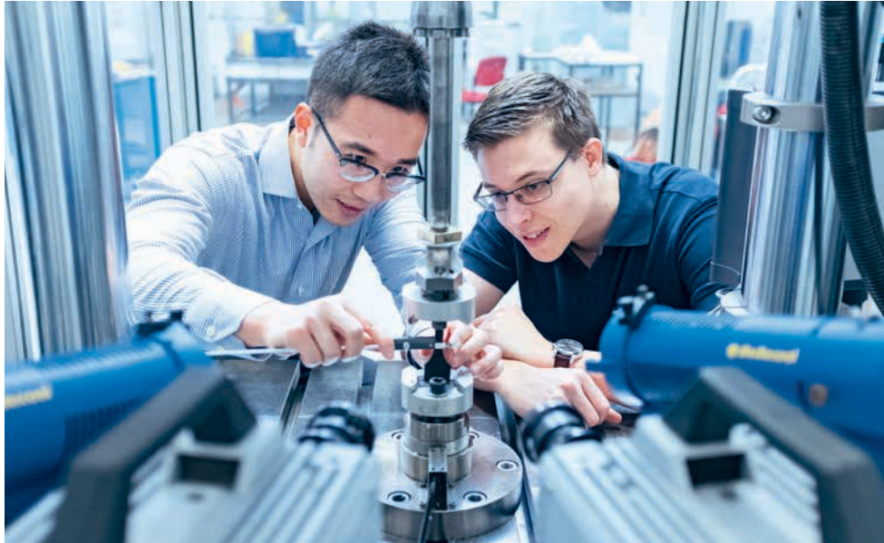
The Department of Lightweight Vehicle Construction at the University of Siegen has a state-of-the-art high speed testing machine. This is used to test the tensile properties of new plastics developed as part of the project at high strain rates. Doctoral student Danshi Li from the University of Siegen and Adrian Baur from Röchling Automotive insert a new material sample in the machine.
